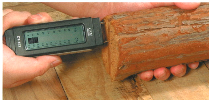
Measuring dampness in Timber
