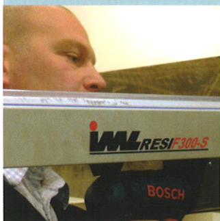
Resistograph drilling in progress
